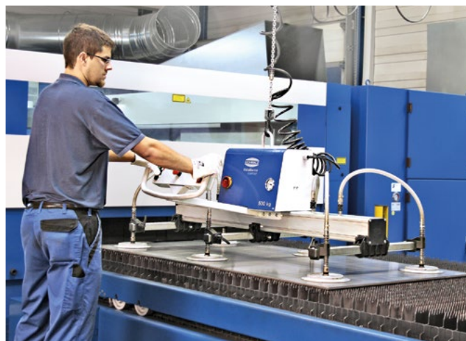
Vacuum lifting device VacuMaster Comfort for loading and unloading a laser cutting machine
