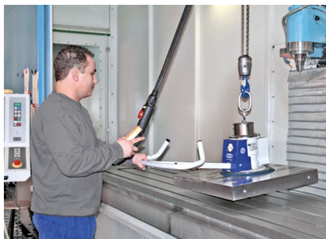
Vacuum lifting device VacuMaster Eco for energy-independent handling metal parts
