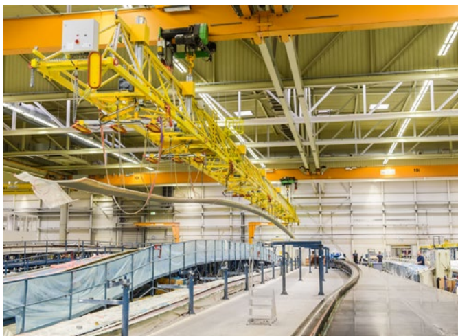
Wind energy | Vacuum lifting device VacuMaster for GRP components in rotor blade manufacturing weighing several tons and up to 60 m in length
