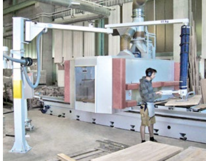
Articulated-arm jib to move around obstacles
