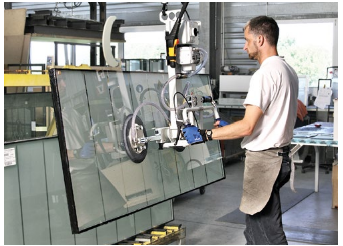
VacuMaster Window for vertical handling of glass elements
