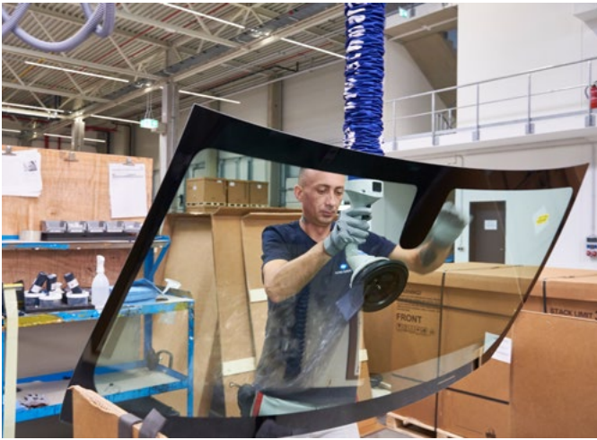
Vacuum tube lifter JumboFlex for handling windshields
