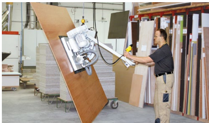
VacuMaster Multi for swiveling wooden boards by 90°
