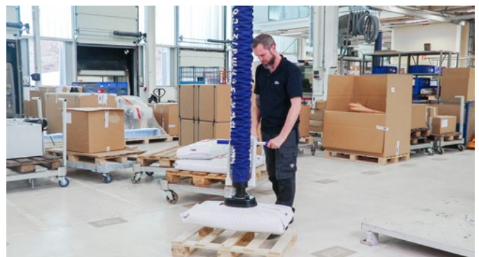
JumboFlex High-Stack when handling bags
