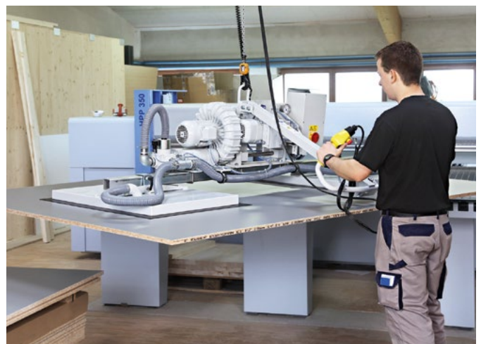
Vacuum lifting device VacuMaster Multi with 90° swivel angle for handling heavy, porous wooden boards
