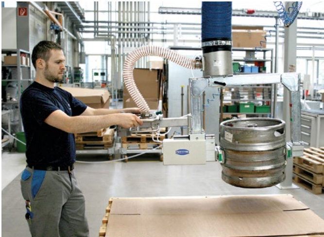
Beverages | Vacuum tube lifter JumboErgo with mechanical pneumatic grippers for lifting and turning kegs
