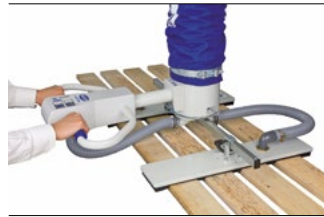
Vacuum area gripper FMP For pallets, sections or cut pieces where the vacuum gripper is not fully covered by the workpiece. The grippers can be continuously adjusted along the beam.
