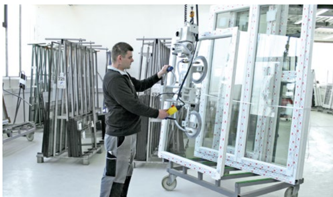
VacuMaster Window for rotating and palletizing windows
