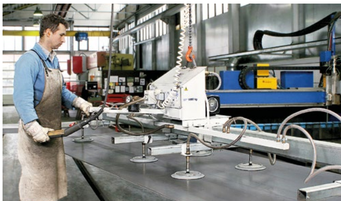
VacuMaster Vario in process of loading and unloading a laser cutting machine
